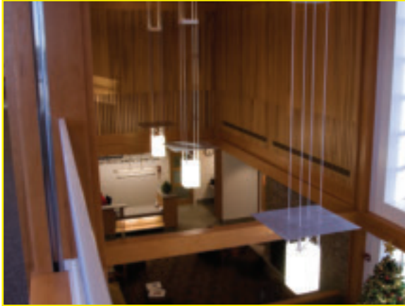
The main lobby features custom-made hanging fixtures that add a touch of elegance to welcome patients. These fixtures are used in other waiting rooms, too. Note the reflectors that provide indirect lighting.
