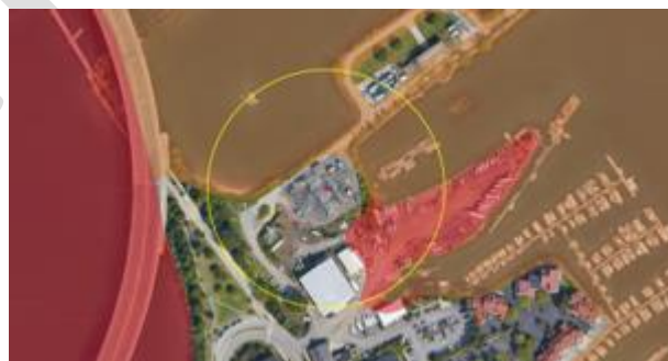
Figure 22. Cape 115 kV Substation overlaid with FEMA's 100-year coastal and inland floodplains
