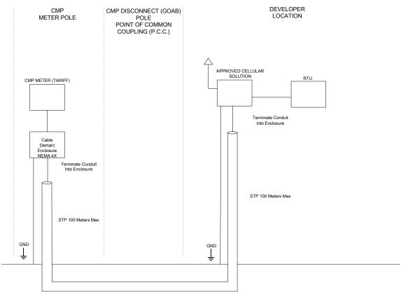
UNDERGROUND CONDUIT - Minimum 24" below ground level
