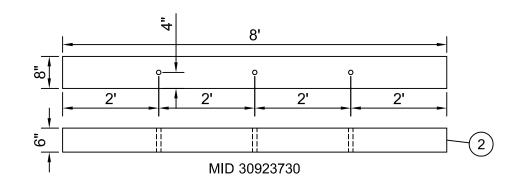
NOTE A: UNDERCUT THE HOLE TO GET THE ENTIRE ANCHOR BEARING AGAINST UNDISTURBED EARTH.
