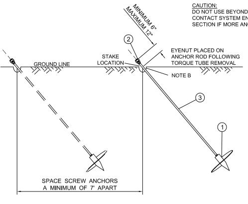
DO NOT USE BEYOND TWO ANCHOR EXTENSIONS (14 FEET). CONTACT SYSTEM ENGINEERING - TRANSMISSION SECTION IF MORE ANCHOR DEPTH IS REQUIRED.
