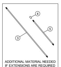
NOTE A: THE ANCHOR ROD SHALL BE SET IN ALIGNMENT WITH THE GUY STRAND. REFER TO THE STRUCTURE GUYING DETAIL ON THE PLAN & PROFILE TO CALCULATE GUY ANGLE.
