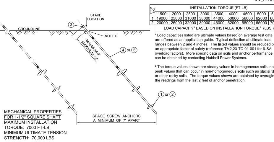
NOTE A: THE ANCHOR ROD SHALL BE SET IN ALIGNMENT WITH THE GUY STRAND. REFER TO THE STRUCTURE
