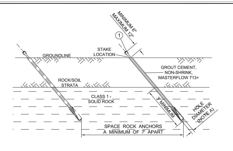
NOTE A: BORE HOLE BY HAND OR WITH POWER DRILL. DIAMETER OF HOLE TO BE EQUAL TO DIAMETER OF UNEXPANDED BOLT PLUS 1/8" (2-3/8" DIAMETER HOLE FOR 1" ROD & 2-1/4" ROCK ANCHOR).
