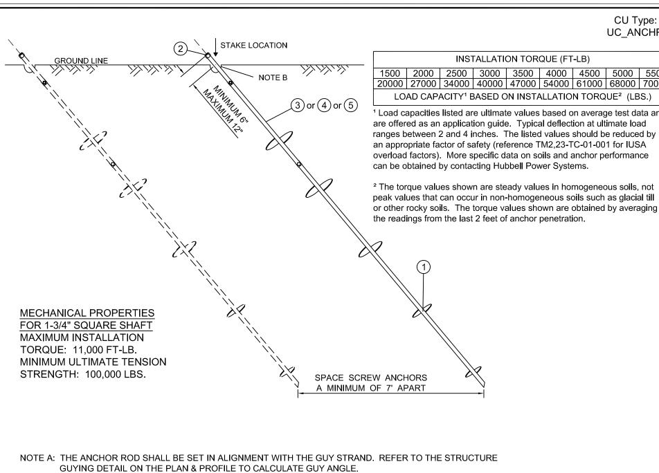
NOTE B: DIG A SMALL HOLE AT THE ANCHOR ENTRY POINT TO PREVENT "WALKING".
